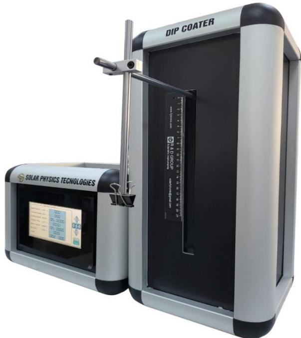
Dip-coating process is one of the commonly used liquid-phase deposition method for the formation of thin films. The technology of this process is based on dipping a substrate into a solution at a controlled rate. After the liquid component of this solution is dried, a solid thin film is remained on the substrate. Thus, the importance of the adhesion and cohesive forces between the dipped substrate and the solution is relevant in the process.
